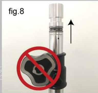
Unpack the vertical stand tube assembly. WARNING: Smaller tube under pneumatic pressure. DO NOT loosen height adjustment knob until the stand is completely assembled or risk injury. (fig. 8)
