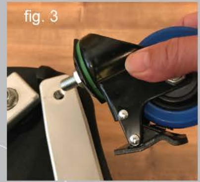
Thread and tighten caster mounting bolt in the hole in each leg. (fig. 3)
